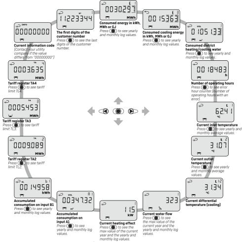
Display readings are based on **DDD-code 310 /610**. At kamstrup.com, you can find a selection of interactive user guides based on other DDD-codes.
